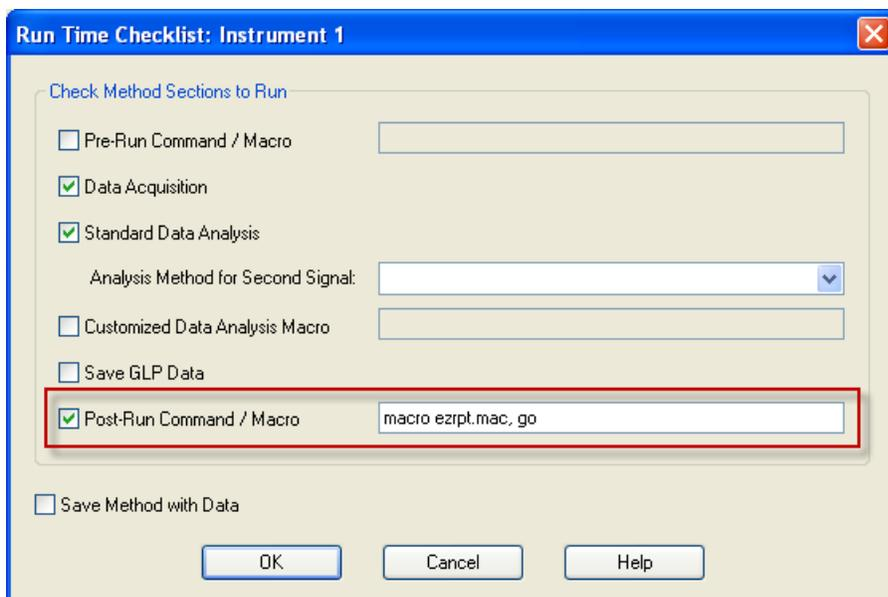
The Agilent ChemStation “Run Time Checklist” dialog box configured to send results automatically to the EZReporter software at the end of each run.
