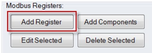
Note: The Modbus Slave Server must be stopped before you can make changes to the Modbus configuration. If the server detects that a Modbus Master is connected, you will be prompted whether or not you want to continue. If you stop the server with a Modbus Master connected, the Master will experience errors since the Slave will no longer respond.
