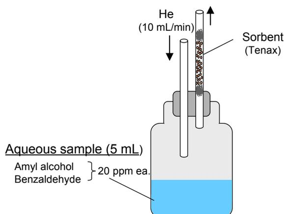
Figure 1. Trapping volatiles with sorbent
