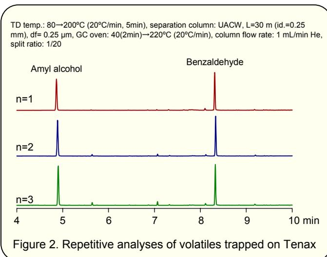
Figure 2. Repetitive analyses of volatiles trapped on Tenax
