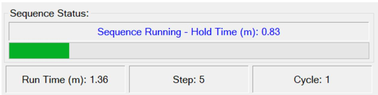
When a sequence is running, the run time, step number being executed, and the current cycle are displayed. In addition, if a HoldPosition step is being executed, a hold-time progress bar will be displayed.
