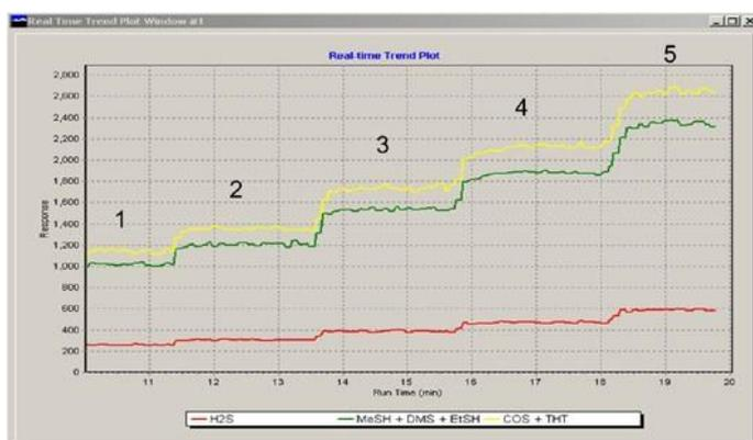
Figure 14: Monitoring stepwise changes in low-level sulfur gases: Step 1: 1.0 ppm (mercaptans) to Step 5: 4.0ppm (mercaptans).
